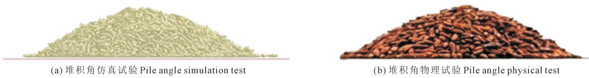
图 8 沙棘籽堆积角仿真试验与物理试验 Fig.8 Simulation test and physical test of sea buckthorn seed accumulation angle
