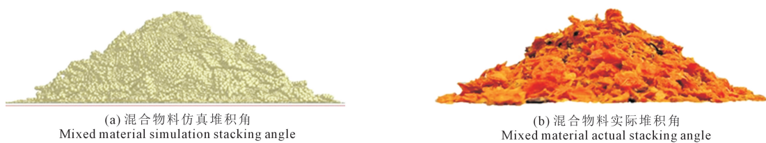
图 11 沙棘籽-果渣混合物堆积角试验与仿真 Fig.11 Test and simulation of stacking angle of sea buckthorn slag and seed mixture
